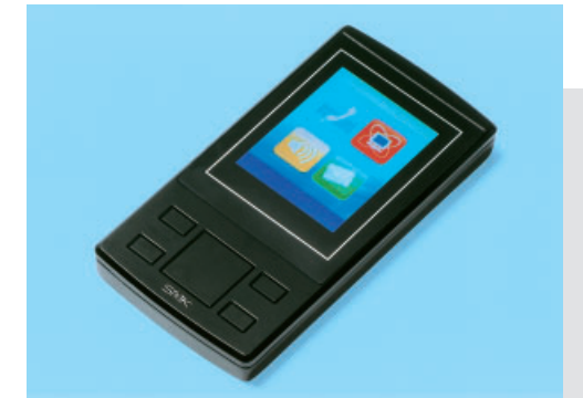
for mobile equipment The force feedback (FFB) touch panel
